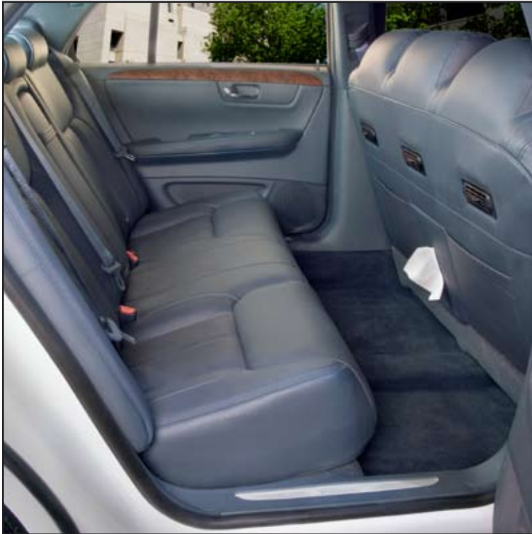
Center seat design provides additional foot room for rear seat passengers.
